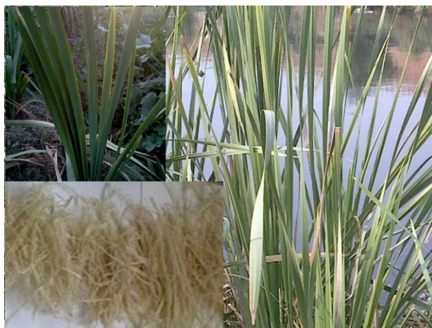
Figure 1. Collection of lignocellulose fibers from stem of T. Angustifolia plant. [Color figure can be viewed in the online issue, which is available at wileyonlinelibrary.com .]
